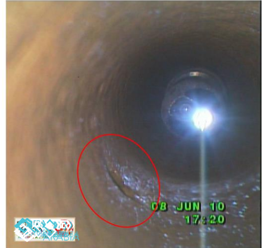
This picture (waveform on the left) shows tagged area of the signal response from internal corrosion indicating 35-40% ID LWL detected in A-179 fin-fan (air cooler) tube, that corresponds with boroscope picture on the right
